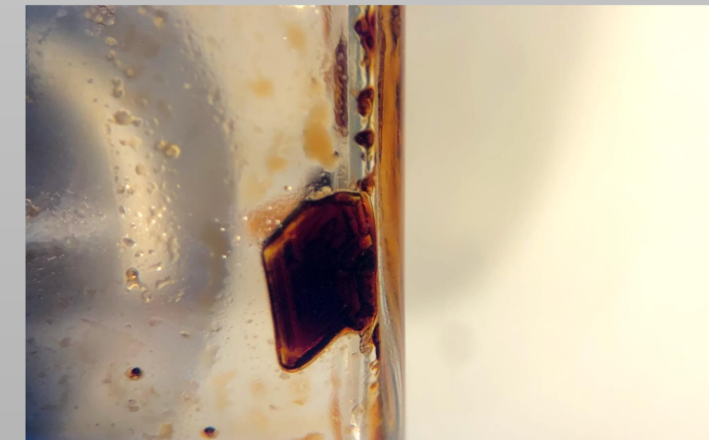
NHC-Mn(CO) 5 Br crystal grown in DCM and Hexane vial. Sent for further analysis.
